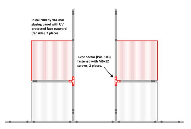
■= M6x12 mm screw loaded in a previous step
