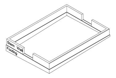
Concrete stem wall foundation with door openings
