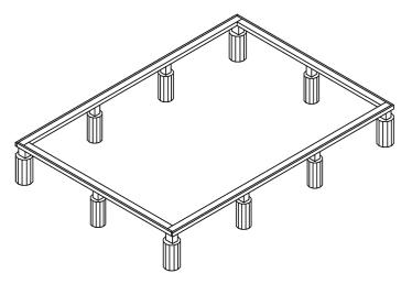
Pier and beam foundation with piers set in concrete below grade
