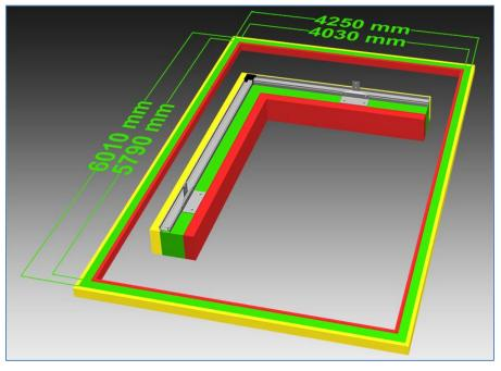
The overall substrate dimensions are the combination of several dimensions. Only the overall greenhouse dimensions are specified by the manufacturer. You must calculate the others.
