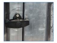
The spring side fits nicely in the deep door slot but it is helpful to partially fill the left door slot for a snug overall fit. Place an extra piece of the aluminum frame material into this slot to take up the slack. You should drill a hole in this filler to clear the head of the Phillips pan head screw (Pos. 142) that secures the crossbar to the vertical profile.
