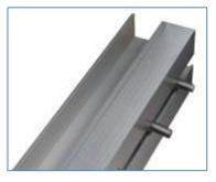
The M6 screws are loaded into capture slots in the various profile extrusions. All of these slots, and consequently all M6 screws, face the interior of the greenhouse. The M6 screws are loaded into the slots from the open ends and should therefore be loaded before the profile is secured in place. Loading a screw after the profile is in place is inconvenient and may require some disassembly.
