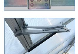
The opening temperature is controlled by the distance you thread the cylinder into the yoke. Fully threaded, the window will open at the minimum temperature. Thread the cylinder farther out (anti clockwise) to raise the opening temperature.
