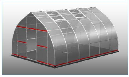
Seal the bottom edge of every glazing panel. Mask with Scotch Blue painter's tape to form a bead on the glazing surface 3 to 5 millimeters wide from the profile edges. Apply the sealant and tool it to slope from glazing surface to profile edge. Allow it to cure for 24 hours before removing the tape.
