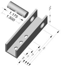
Concept drawing of a taut wire anchor machined from 1-inch aluminum channel
