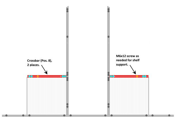
= M6x12 mm screw loaded in this step, 8 places
