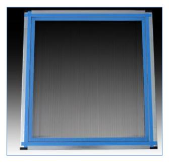
**Press the T-seal into the profile retaining slots on the bottom and both sides of the window.** Do not install T-seal on the top profile. The lip of this profile is part of the hinge that fastens the window to the roof beam.
