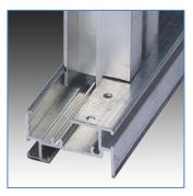
The curved vertical profiles of the side walls are fastened to the floor profiles and to the substrate by the mounting brackets (Pos. 6.7). The vertical profiles of the gable walls are initially fastened to the floor profiles with 4.2 by 13 mm self-tapping Phillips head screws and ultimately by mounting brackets.
