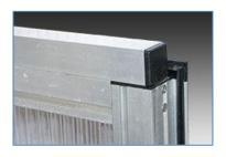
Install the seal in the door's top profile before you attach the rectangular tube. The seal material should extend over the full width of the door, not just the width of the rectangular tube. You can trim it after the door is fully assembled. The pre-drilled holes in the rectangular tube are offset, so it will fit only one way on the top profile.
